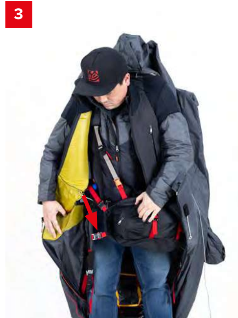
3 Connect the front support pillar metal buckle and adjust the volume of the container with the red straps
