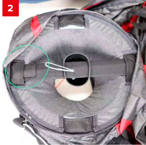
2 Pass a plastic parachord through the white line loop
