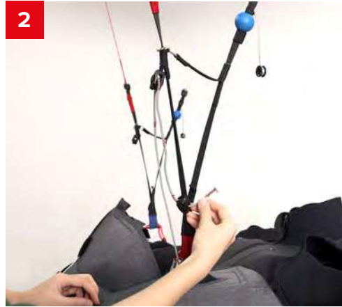
2 After passing it through the top pulley, pass the line through the bottom pulley
