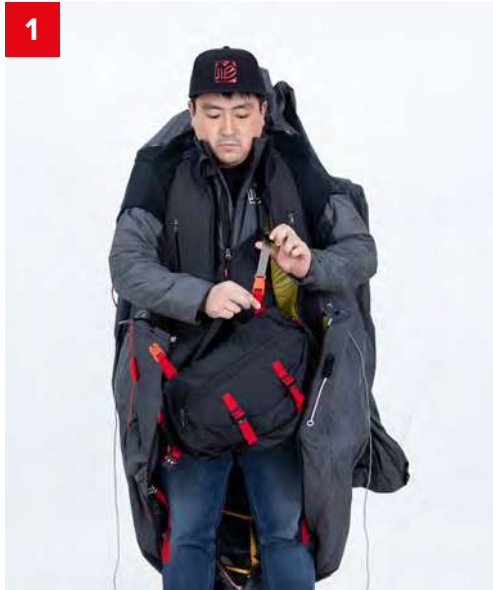
1 Attach the shoulder strap with the orange plastic buckle
